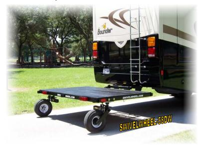
Each Swivelwheel system has its own market, due to the design, deck dimension, and available weight capacities . Regardless of the size, all systems include the same anti-fishtail, anti-jackknife feature. The system can only track with the towing vehicle due to the Dual Point hitch assembly supplied with each product.
