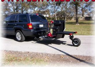
The *Swivelwheel-MOB* system is a new design for 2008. This is the first single wheel transport system designed originally for the mobility industry. We have had numerous requests from customers to order the Swivelwheel-46 system to transport their mobility scooters and/or electric wheelchairs. The problem with the Swivelwheel-46 in that application is the deck height. That system has a 25" deck height which makes it prohibitive for that market.
