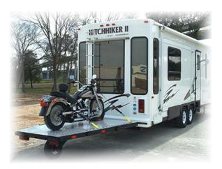
The lift systems that are installed and do not bend the chassis frame, fishtail while driving down the road due to reduced king pin weight. When the combined weight of the lifting device and motorcycle are downloaded to the rear of the trailer, (could be over 1100 pounds or more of direct downward force) it reduces weight on the king pin, thus giving an unstable ride at or below highway speeds. The following is a quote received via a recent email that may sum it all up:
