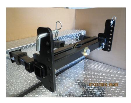
Assemble the Tandem Tow frame and slide it under the SWIVELWHEEL-59DW's frame as shown below and in the engineering drawing.
