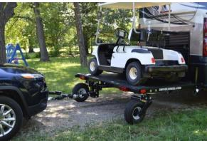
The Swivelwheel-58DW Tandem Tow allows the owners of the SWIVELWHEEL-58DW system the choice to tow a 6000 pound vehicle behind the SWIVELWHEEL-58 platform. This option is not available for the SWIVELWHEEL-58 Single Wheel System.
