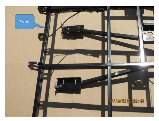
Lift the Tandem Tow frame up to the SWIVELWHEEL-58DW frame and clamp or block into position. With the supplied mounting bolts, bolt the system into place as shown in the following photos below. Once all mounting bolts are in position, tighten all nuts fully.
