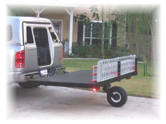
The Swivelwheel-58 may be loaded from the driver side, passenger side, or rear. The system retains most of the features of the original design, while adding other unique qualities.
