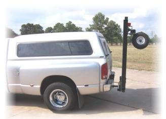
The Cruiser Ramp Electric Motorcycle Loader may also be incorporated into the Swivelwheel-58 system. This allows the motorcycle to be pulled onto the deck without riding up ramps.
