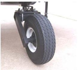
The tire is a  $5.70 \times 8''$ , D-Rated, 8-Ply, Highway Speed Trailer Tire. The load rating with this tire is 1075 pounds @ 100 psi cold inflation. This tire will never see 1075 pounds at a 1000 pound deck load.
