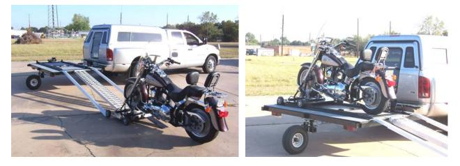
Front Jack Stand Legs are provided with the system so that the swivelwheel-58 may be moved around while detached from the tow vehicle. These legs are removable for storage. You don't have to find someone to help lift the front of the product to roll it away.
